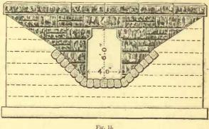
to prevent any undermining by the stream or upheaval by frost.
